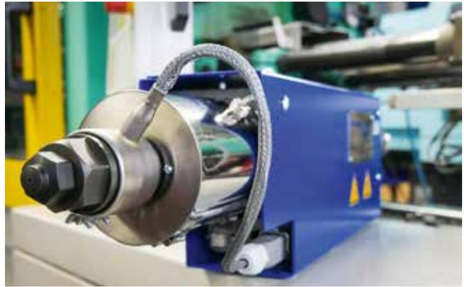
Fig. 3. Energy-efficient inmex plasticizing unit for an Arburg injection molding machine (© inmex)
