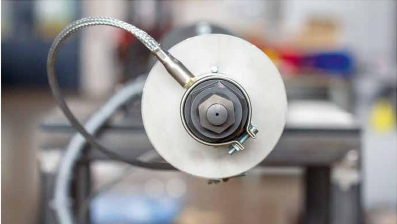
Frontal view of an inmx plasticizing unit. Not visible from the outside: the heating elements integrated into the barrel (© inmx)
